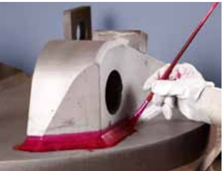
Dye penetrant test
